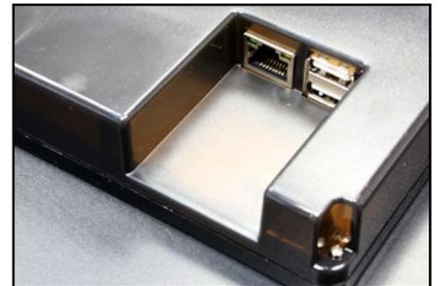
Figura 3 - 2 Puertos USB host y Puerto Ethernet
