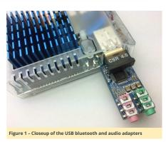
Insert the USB Bluetooth and audio adapters into available USB ports on the ODROID-XU4, then insert the headset's headphone and microphone plugs into the corresponding jacks on the audio USB adapter.
