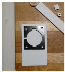
Figure 1 – I just set the little board over my cut panel and marked it with a sharple  $\,$
