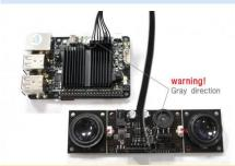
Figure 5 – Attaching the Stereo Boom Bonnet to an ODROID-C1+/C2
