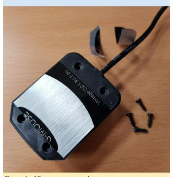
Figure 4 - All screws removed
