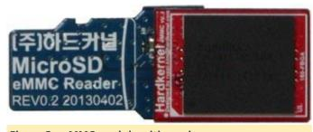
Figure 3 - eMMC module with reader
