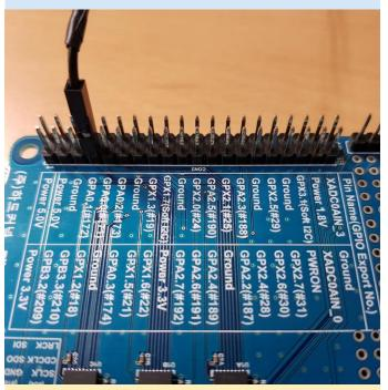
Figure 10 - PPS pin attached to XU4
