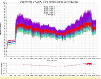
Figure 3 - Dual Mining GPU/CPU Core Temperatures vs. Frequency
