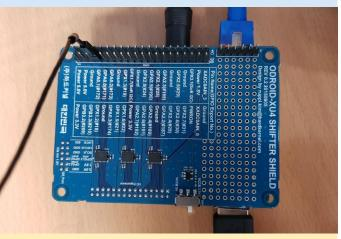
Figure 11 - Pin and USB connected to XU4
