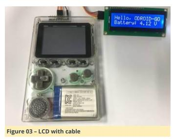
Let us learn how to use I2C interface on the ODROID-GO IO expansion port. First, you will have to connect the 16×2 LCD to your ODROID-GO's P2 (expansion connector) as follows:
