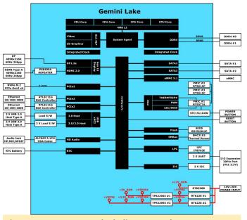
Figure 2 – ODROID-H2 Block diagram and interconnections.
