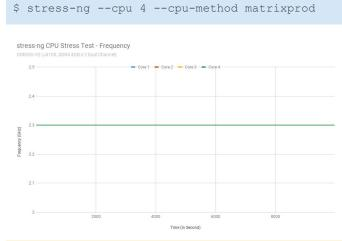
Figure 6 - ODROID-H2 CPU stress test results
