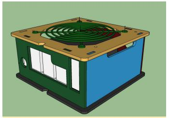
Figure 16 - Design prototype for ODROID-H2 case
