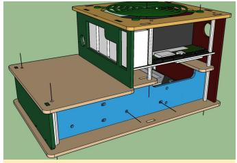
Figure 23 - Design prototype for ODROID-H2 case
