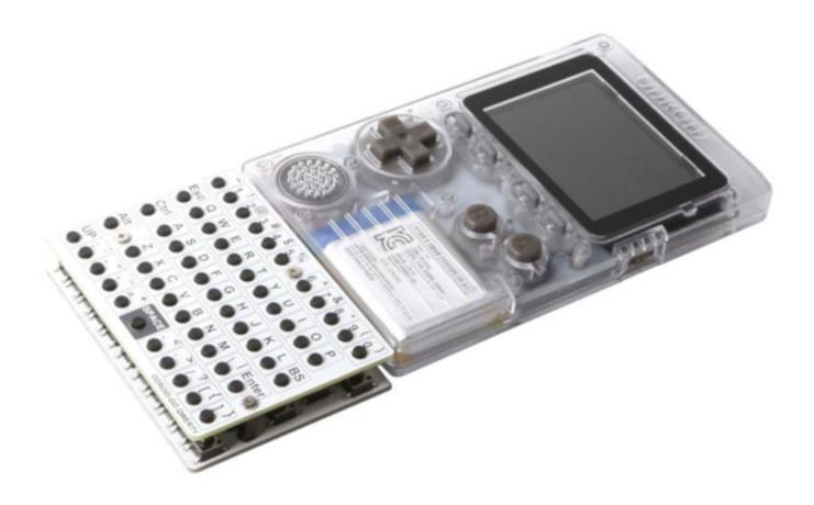
With Hardkernel's new bluetooth keyboard, you can You can also type in and run BASIC language turn your ODROID-GO to a portable handheld computer. ODROID-GO can emulate some classic computer systems such as Commodore 64, ZX Spectrum, and MSX. We believe a physical keyboard provides a better emulation experience for these systems.
