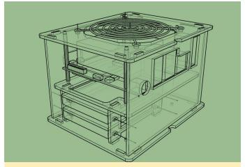
Figure 20 - Design prototype for ODROID-H2 case
