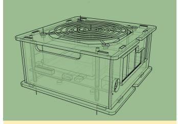
Figure 17 - Design prototype for ODROID-H2 case
