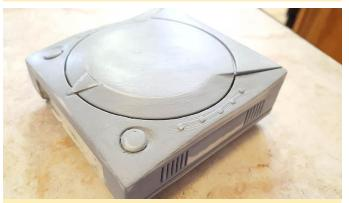
Figure 13 - We had to drill a small hole through power button stem so we could secure with a paperclip
