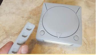
Figure 14 – We had to drill a small hole through power button stem so we could secure with a paperclip
