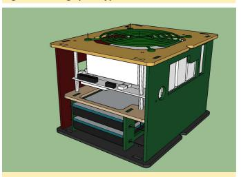
Figure 19 - Design prototype for ODROID-H2 case
