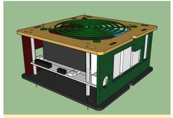
Figure 15 - Design prototype for ODROID-H2 case
