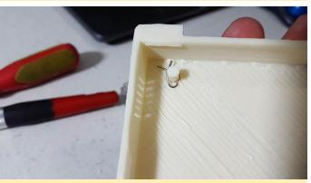
Figure 12 – We had to drill a small hole through power button stem so we could secure with a paperclip
