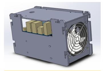
Figure 11 - Design prototype for ODROID-H2 case
