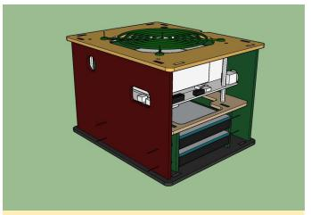
Figure 18 - Design prototype for ODROID-H2 case
