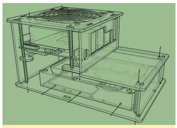
Figure 24 – Design prototype for ODROID-H2 case
