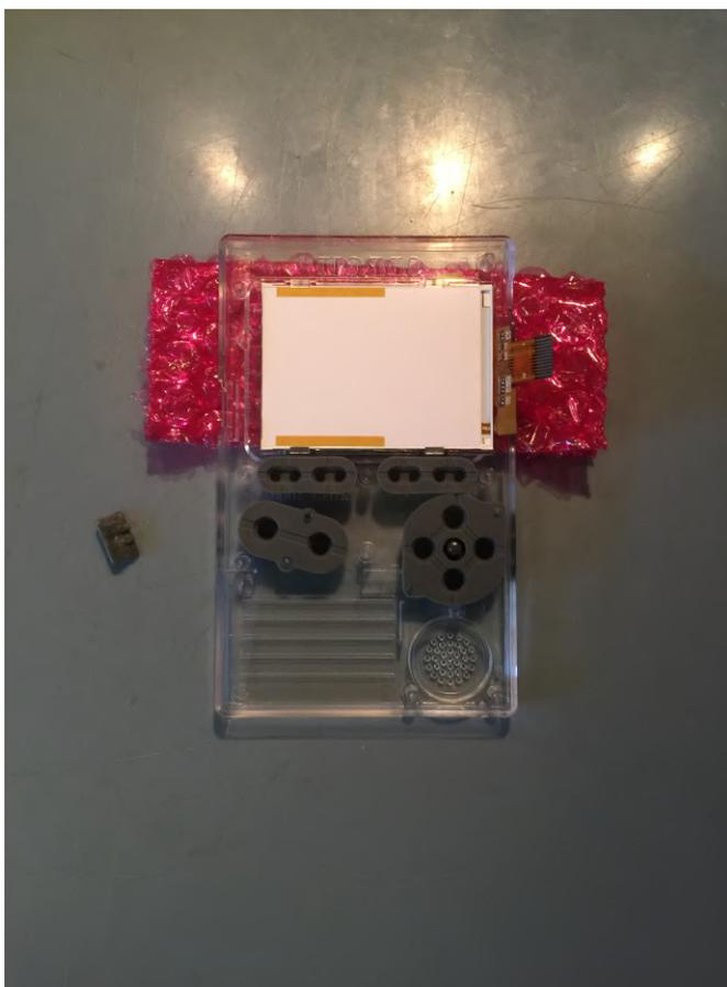
**Figure 4 - Set the button in the slots, making sure they go all the way in**
