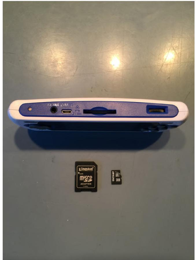
**Figura 2 - Lector USB tarjetas SD/micro SD**
