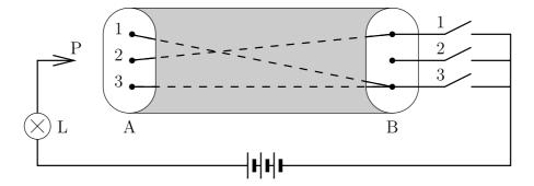
Fig. 1. Cable with three wires and three switches.
