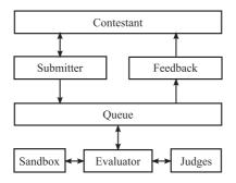
Fig. 1. Typical interconnection of modules.
