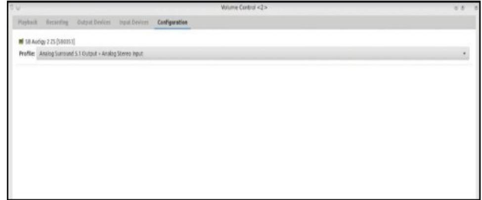
The next important setting is the **Configuration Tab** in **PulseAudio Volume Control** (seen above), where you select your required 'profile' to match your soundcard and speakers.
