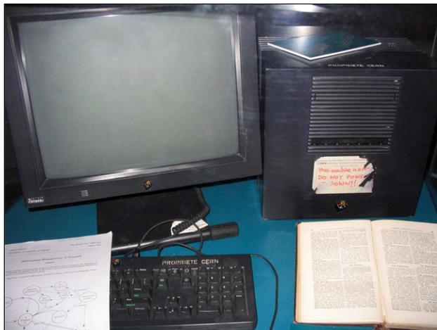
NeXTStep computer used to develop the WWW. Photo: CERN.
