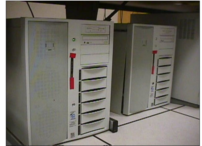
This is the server using only a 300 MHz Dual Pentium II, 512MB of RAM and 9GB of hard drive.
