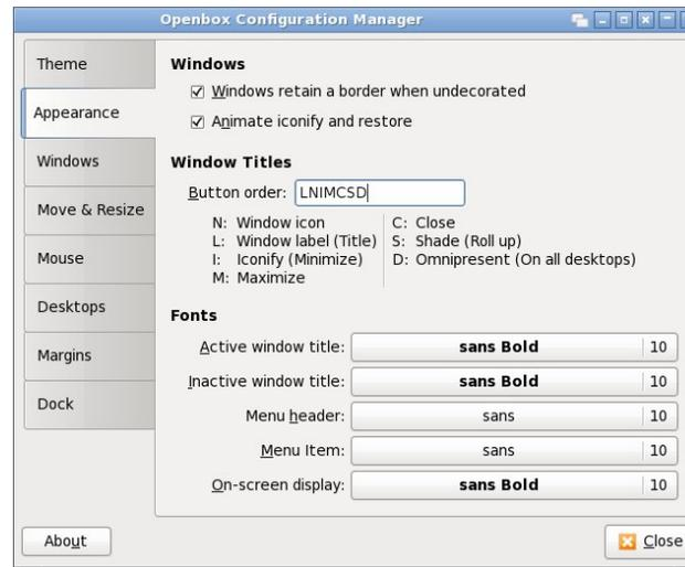
Fig. 04. The Appearance tab, with all the window buttons added. Notice how the window title (L) remains centered - despite being the first variable listed - and is offset only by the other buttons
