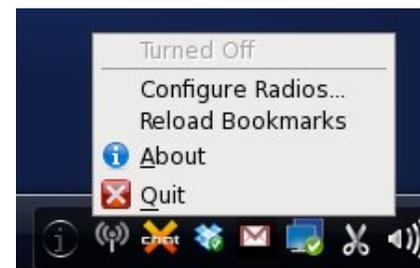
A right click of your mouse button on the Radio Tray icon will display the menu shown above. Selecting "Configure Radios..." from the menu will bring up the configuration dialog box.
