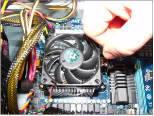
*Installing the CPU cooler atop the CPU.*
