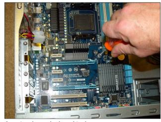
Securing the motherboard in the new case.
