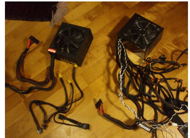
Photo: Modular vs. Non-Modular PSU (courtesy Ni-Sama at Wikimedia Commons)
