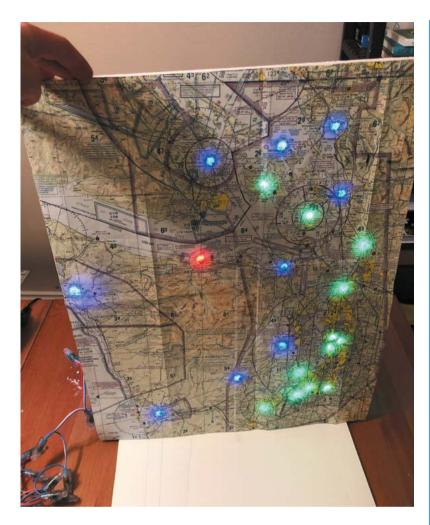
Refinements include making the lights blink if there are high winds at an airport, and another addition to make the LEDs flash white if there is a lightning storm in the area. He's recently added a small LCD which shows full weather information for the airports. In response to feedback by makers on GitHub, Philip added a lightning indicator and set LEDs to blink if a weather station is reporting high winds
