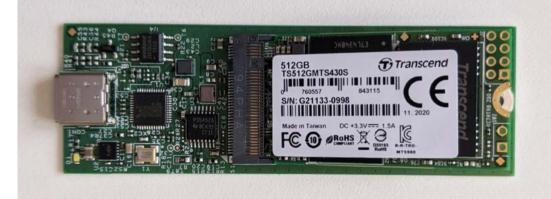
The M.2 SSD adapter translates the SATA III interface on the M.2 SSD drive into a USB-C connection. This is used with a USB-C to USB-A cable to connect the drive to the blue USB 3.0 connection on Raspberry Pi 400
