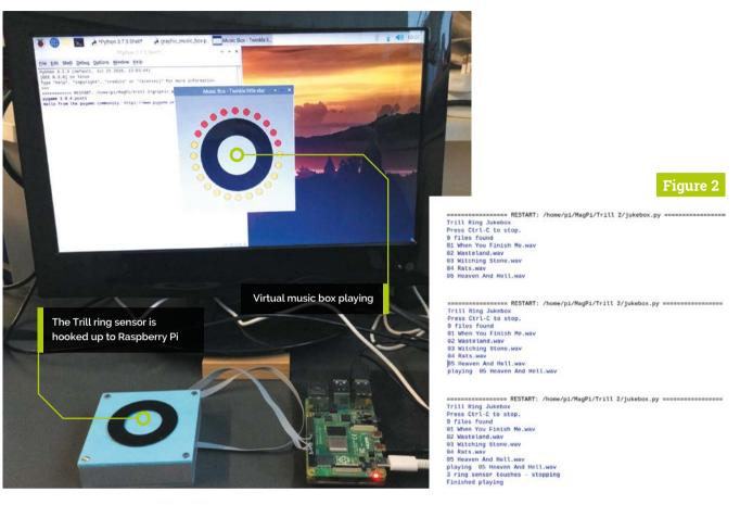
Finally, by adding a ring sensor to the square sensor, you can emulate a scrolling centre button mouse - see the code trill\_simple\_mouse\_scroll.py for how to do this.
