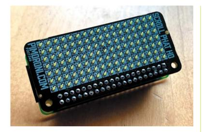
The Scroll pHAT HD without its diffuse 119 very bright LEDs Enter the code from **busybot.service**. (Change the paths if you've created the code elsewhere.) Save the file (CTRL+X and then Y), then enter these commands:
