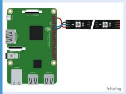
**02** Attach LEDs to Raspberry Pi Zero W and use the code on GitHub to match up lights with your chosen METAR locations.
