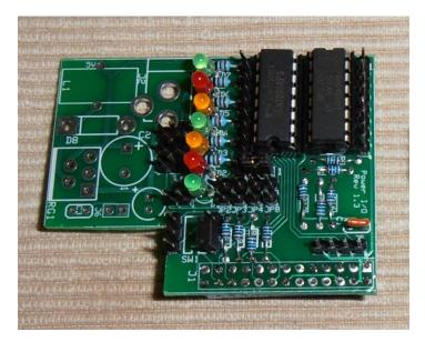
A hexadecimally encoded switch (SW1) can be included if the intended application appreciates its functional or educational value but it has been omitted from the unit pictured above for budgetary or functional reasons, replaced by a pair of 3-pin headers that can be jumpered to match user requirements.
