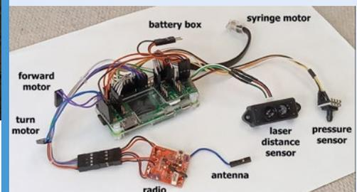
**01** As well as a food syringe and LEGO gear wheels, you'll need a Raspberry Pi Zero 2 W with 16GB microSD card, a LEGO EV3 Medium motor with tachometer, and a 27MHz radio controller.
