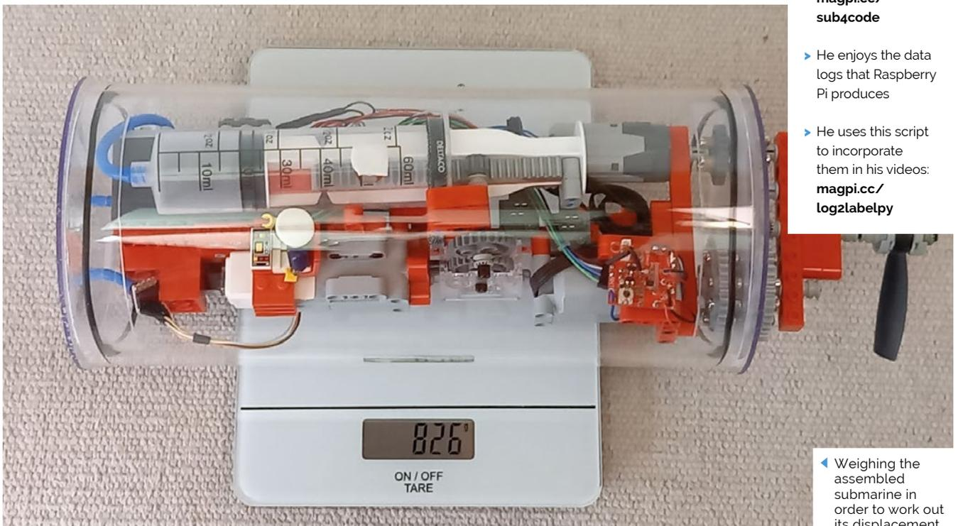
◀ Weighing the assembled submarine in order to work out its displacement
