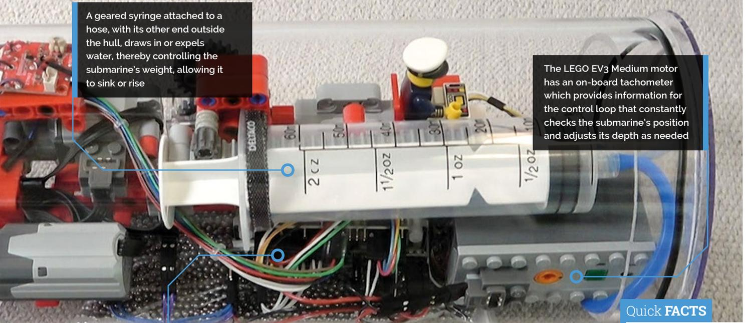
A geared syringe attached to a hose, with its other end outside the hull, draws in or expels water, thereby controlling the submarine's weight, allowing it to sink or rise
