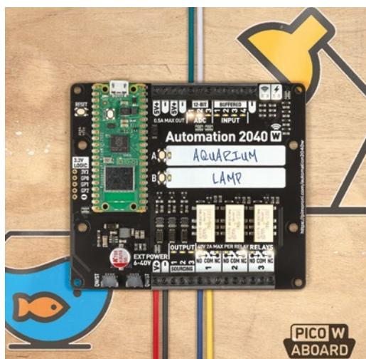
► The Automation 2040 W has a wide range of 40V tolerant inputs and outputs
