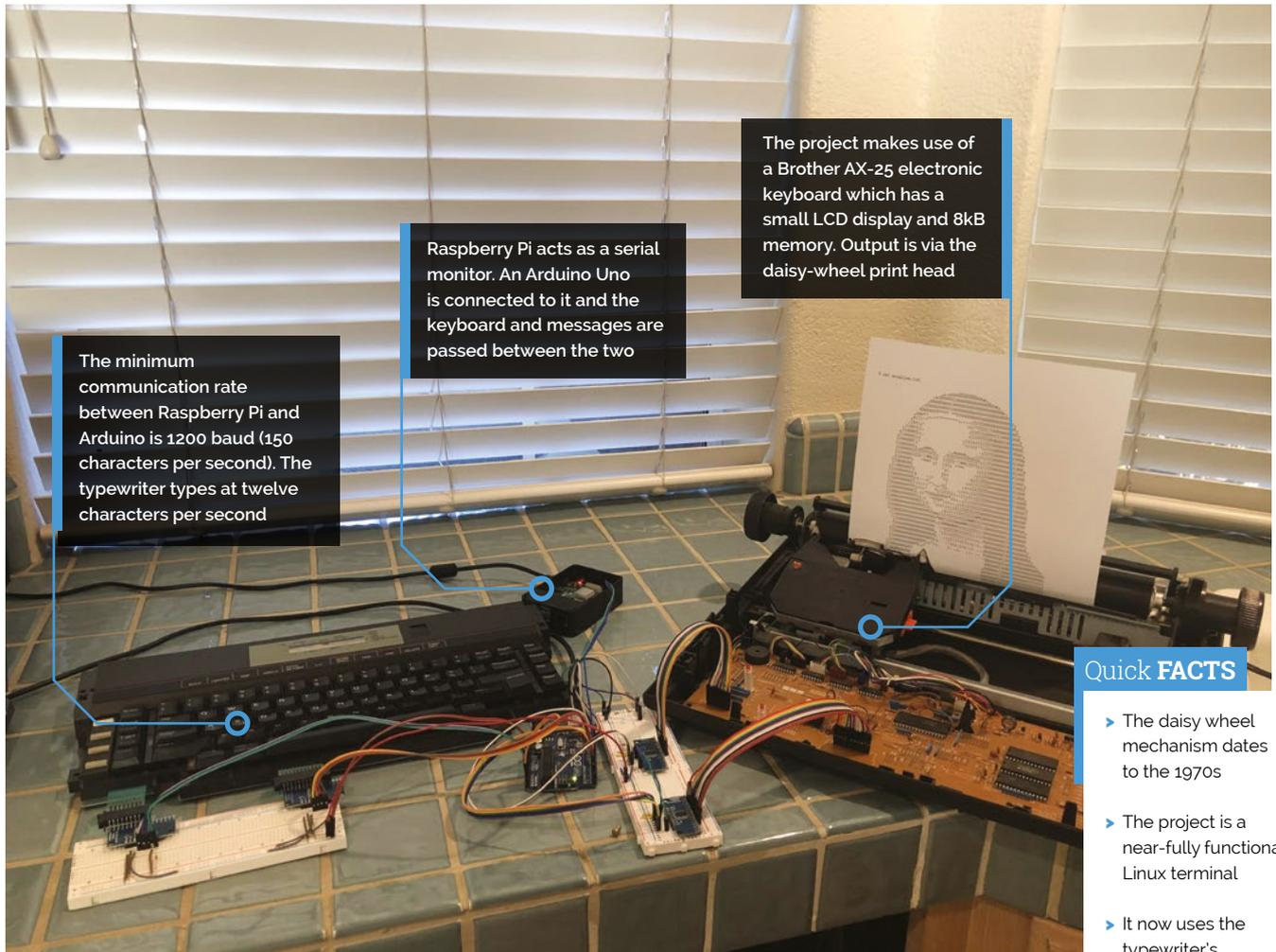
The minimum communication rate between Raspberry Pi and Arduino is 1200 baud (150 characters per second). The typewriter types at twelve characters per second
