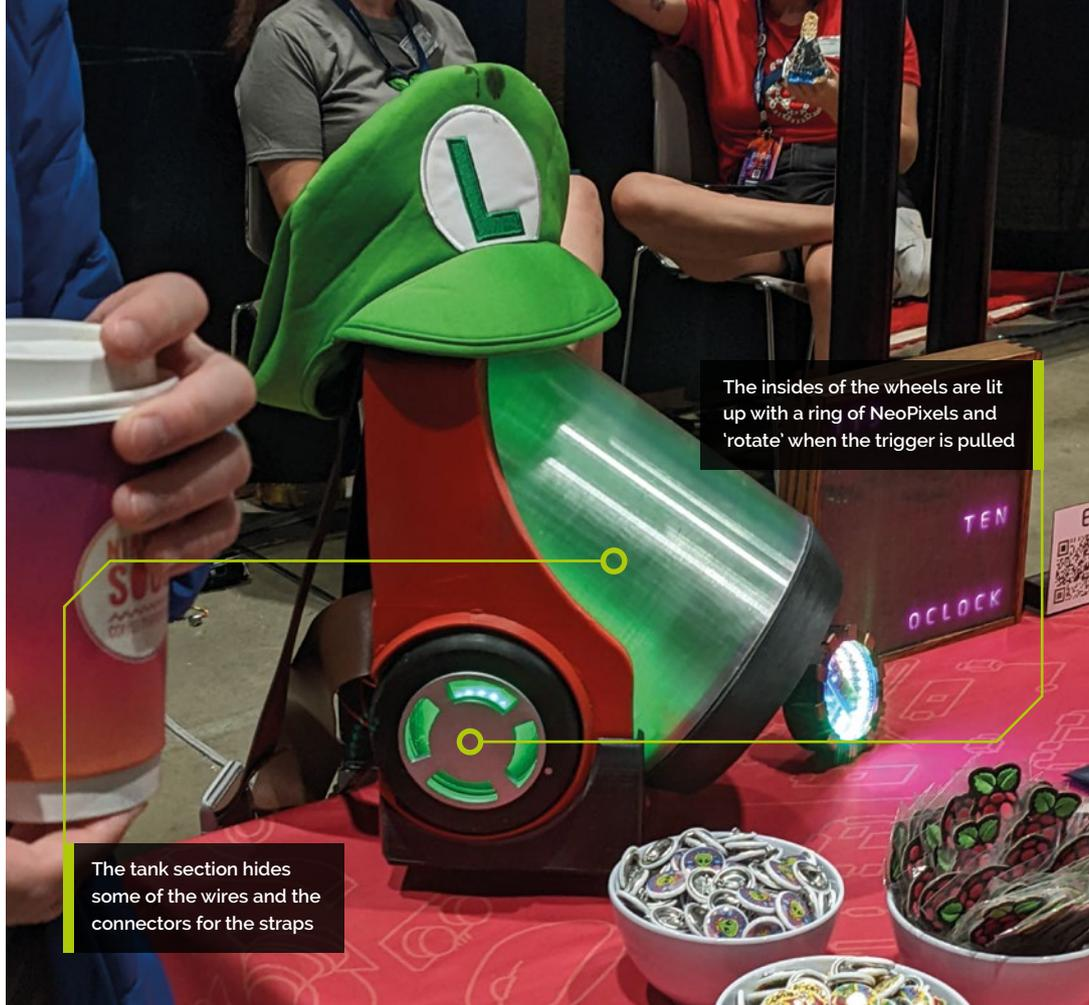
The insides of the wheels are lit up with a ring of NeoPixels and 'rotate' when the trigger is pulled
