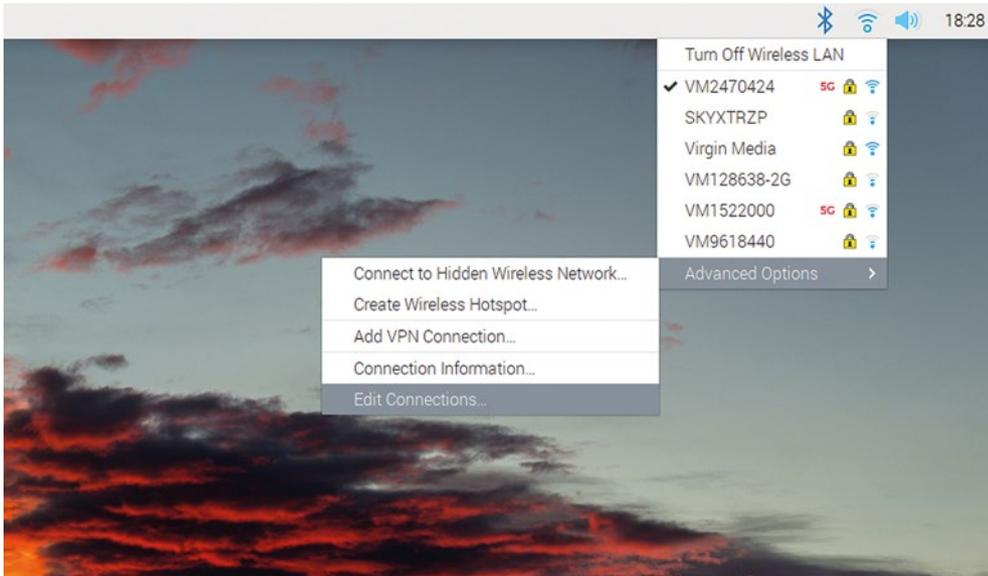
have made any customisations to a wired connection, such as setting a static IP address, you will need to redo those customisations under NetworkManager. (Most of these settings can be accessed via the connection editor, accessed from the ‘Edit Connections’ option in the Advanced Options sub-menu.)
