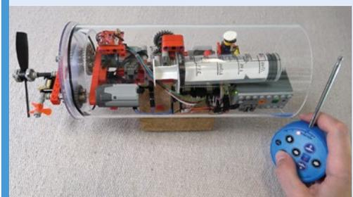
**03** A radio board and controller culled from a cheap toy provide a user-friendly remote control, powered by Raspberry Pi, with no need for a dedicated battery.
