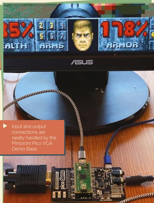
▶ Input and output connections are neatly handled by the Pimoroni Pico VGA Demo Base
