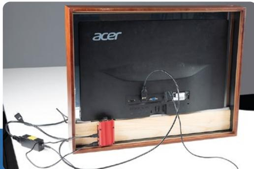
◀ The wood at the bottom helps fill in the space and raise the monitor up, and right-angle connectors help keep the whole system flat to the wall
