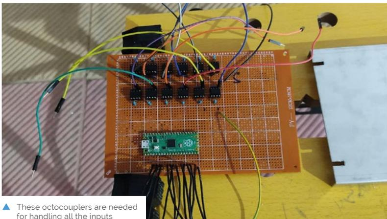
▲ These octocouplers are needed for handling all the inputs
