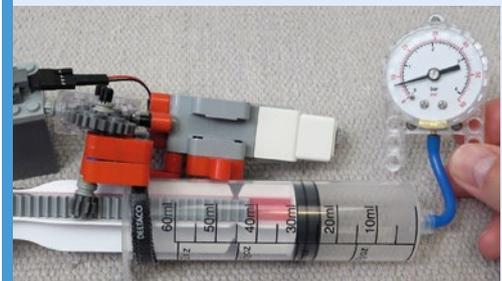
**02** A motorised LEGO gearing system adjusts the ballast syringe. A hose sucks in water and draws water into the syringe chamber. Buoyancy remains constant while the extra weight of water increases the gravitational pressure.
