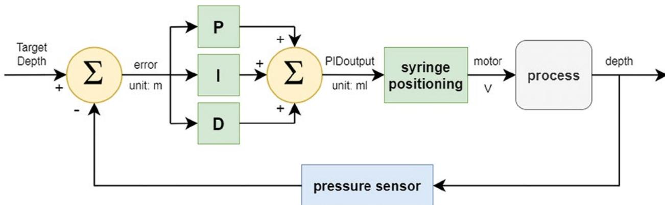
▲ Raspberry Pi's PID control loop takes depth information from the sensors and uses it to adjust the syringe ballast
