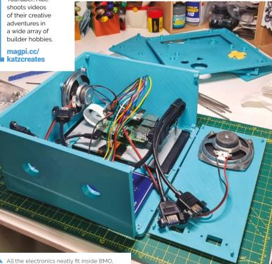
server for remote access, and that is exactly what he is," Allie explains to us. "BMOctoprint is a life-sized replica of the beloved cartoon robot, powered by a Raspberry Pi 4, in a fully 3D-printed case, with functional buttons and a touchscreen face. He can basically control your 3D printer, whilst also giving you compliments and making you laugh, which officially makes him the best 3D printer server ever."
