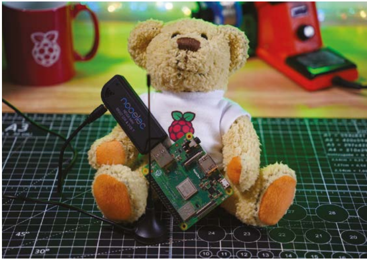
▲ Babbage holds the completed Raspberry Pi board and dongle setup. The antenna is used to detect transponder signals
