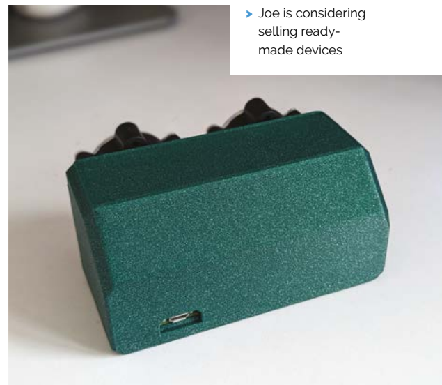
▲ Joe printed his case using a Voron 2.4 3D printer using glitter filament, allowing enough space for wiring and room for a charging port
