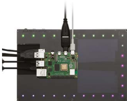
▲ You can mount a Raspberry Pi on the rear of the display using the supplied screws
