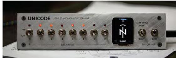
This Pico-powered device is a cool way of displaying unicode using physical switches. It then shows what that arrangement makes and how to create it on a keyboard. Very cool.
