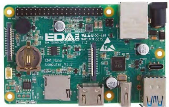
▲ After removing four screws to open the case, you can view the board and access a hidden USB-C port
