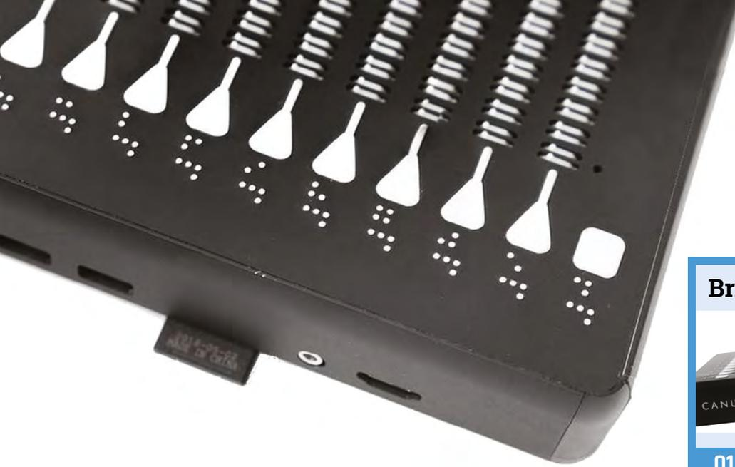
Raspberry Pi Zero is connected to media ports on the main circuit board, and is able to read the BRF (Braille Ready Files), interpret them as Braille, and send them to an Atmel chip on the main board to convert into dot patterns. Each Braille cell is made up of six dots which can either be up or down. There is virtually no margin for error, and a stuck dot can change the entire meaning of a word.
