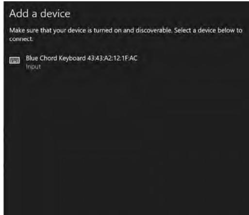
**Figure 10** ♦ The keyboard generates a different Bluetooth address each time it starts
