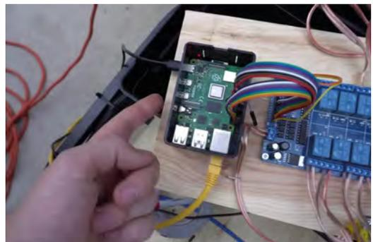
▲ A view of the inner workings, including a Raspberry Pi 4 and relay board
