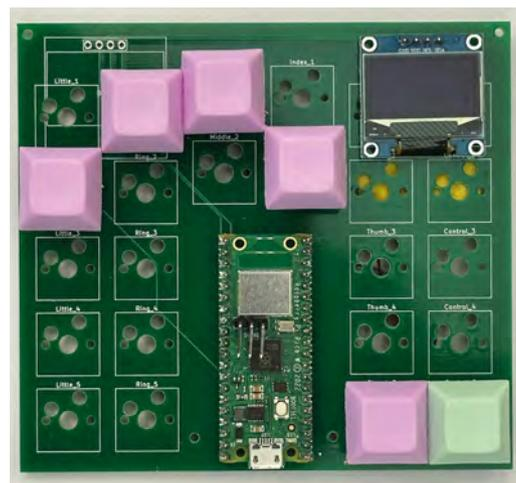
**Figure 5** ♦ The tracks on the top of the board connect the Pico to the display. Tracks on the bottom connect the key switches
