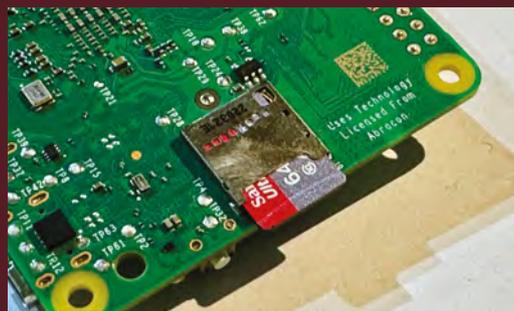
▲ SD cards are very fragile. Insert the card gently into the slot with the gold contacts facing the underside of the board
