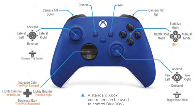
▲ A standard Xbox controller can be used to control BlueROV2
