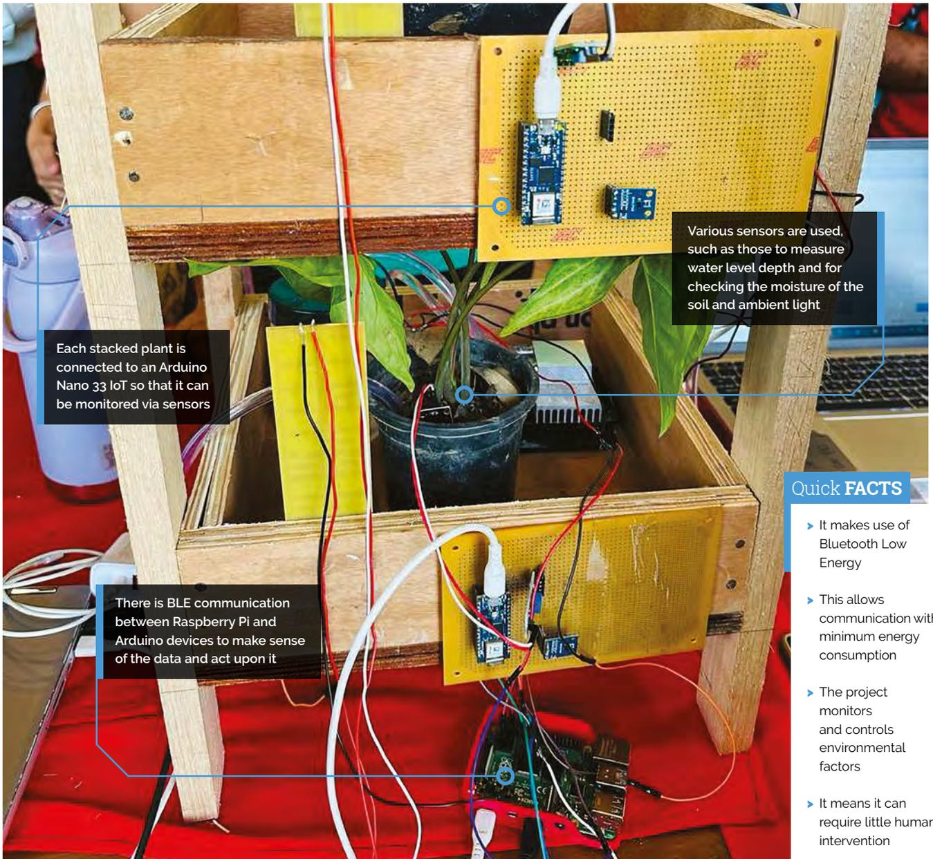
Each stacked plant is connected to an Arduino Nano 33 IoT so that it can be monitored via sensors
