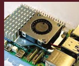
Recent Raspberry Pi models run faster than their older siblings. A Raspberry Pi 5 can work quite safely without any kind of assisted cooling provided, but if you want to get the most speed from it, cooling is useful. There is now the powerful new Raspberry Pi Active Cooler.
