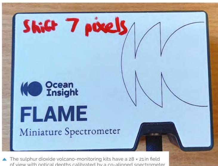
▲ The sulphur dioxide volcano-monitoring kits have a 28 × 21 in field of view with optical depths calibrated by a co-aligned spectrometer
