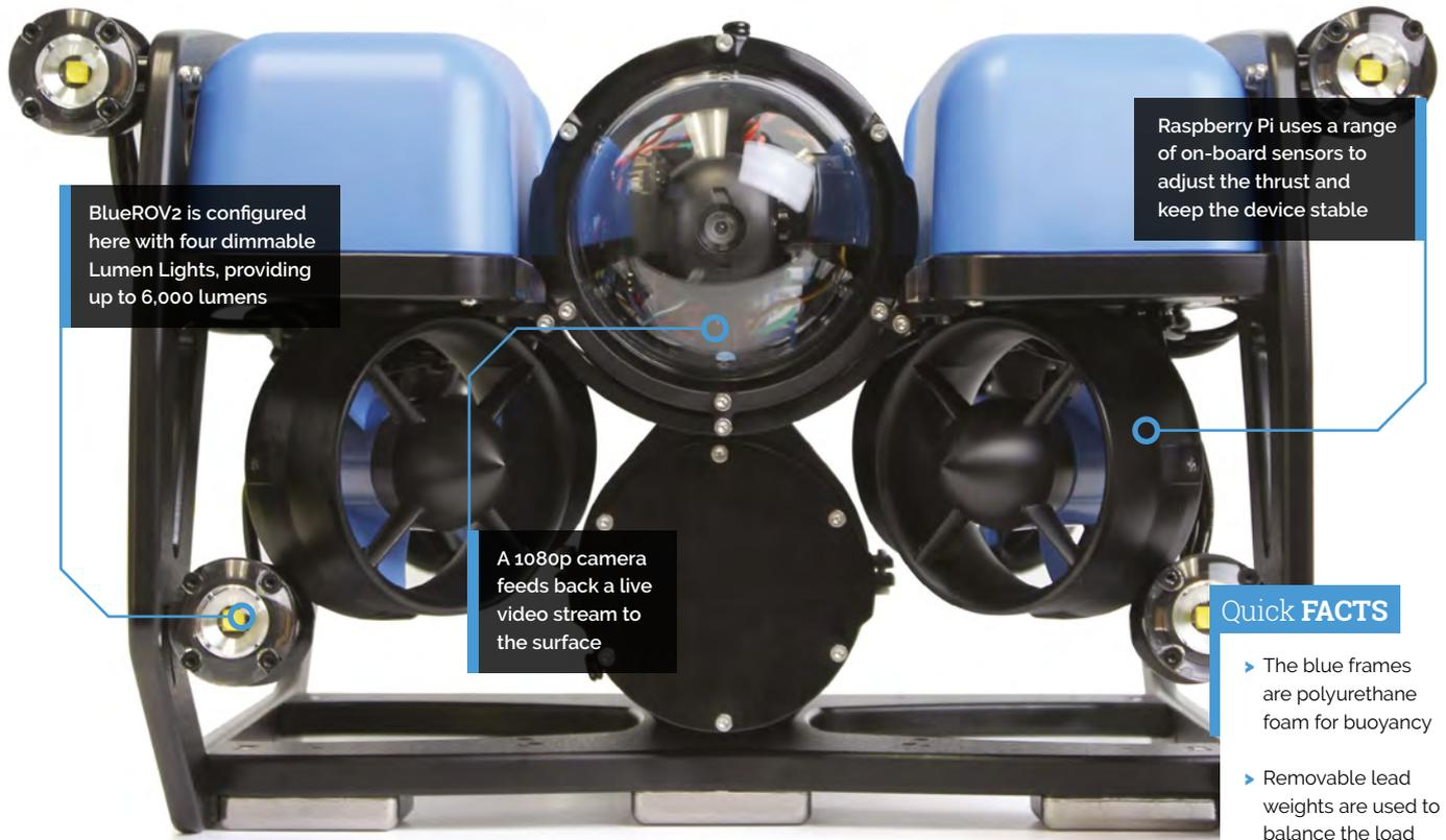
BlueROV2 is configured here with four dimmable Lumen Lights, providing up to 6,000 lumens
