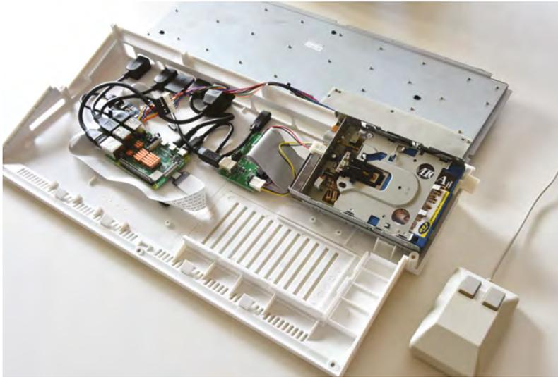
▲ No soldering was needed for this build. The components are simply connected up
