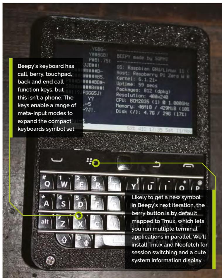
Beepy's keyboard has call, berry, touchpad, back and end call function keys, but this isn't a phone. The keys enable a range of meta-input modes to expand the compact keyboards symbol set
