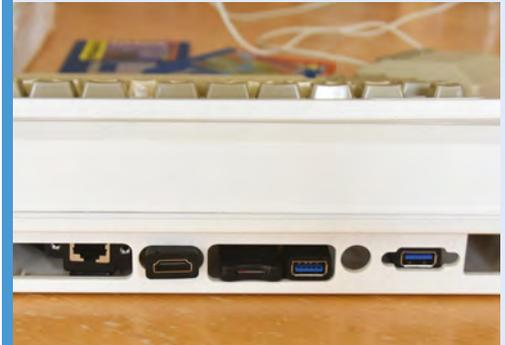
**02** With an assortment of cables, Rob was able to add various ports to the back of the 'Amiga' by ensuring the ends were accessible via the holes. They include HDMI, USB-C, and USB-A, meaning peripherals can be connected to the machine.
