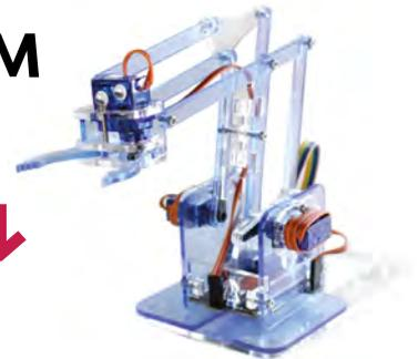
A classic robot designed used in factories the world over, a robotic arm is a nice and simple type of robot where you don't have to worry about locomotion but do have to worry about precise movements and grip. This MeArm kit works with many types of microcontroller as well, and we suspect could also work with Pico with enough jiggery-pokery.
