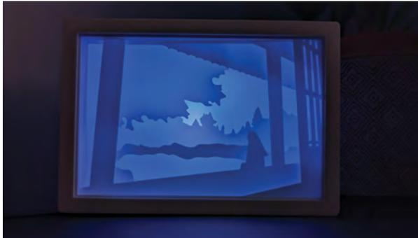
This very pretty box is made up of custom, 3D-printed layers over an 8x8 LED matrix controlled by Raspberry Pi to create excellent vistas.
