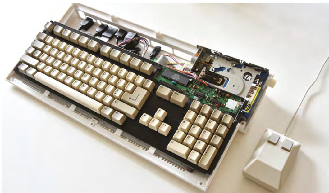
► The Amiga 500 keyboard fits neatly on top of the components with plenty of space available in the case
