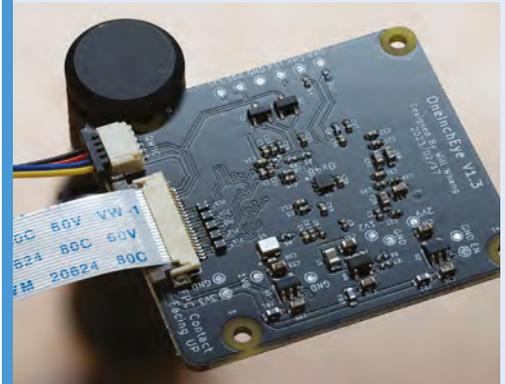
**02** CinePI XL uses a OneInchEye sensor. Code for it is built on top of Raspberry Pi OS 64-bit Lite using libcamera-apps / libcamera. Setup instructions for the original CinePi are at [github.com/CinePi](https://github.com/CinePi).
