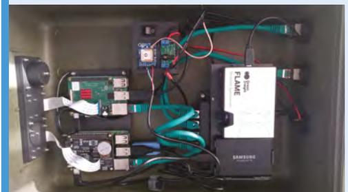
**03** A UV spectrometer, WittyPi HAT, and network drive manage data and send it back to the volcano monitoring team for analysis.
