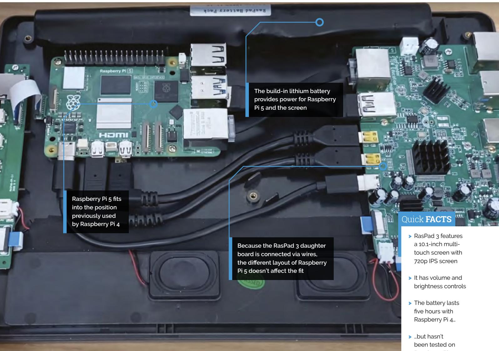
Raspberry Pi 5 fits into the position previously used by Raspberry Pi 4
