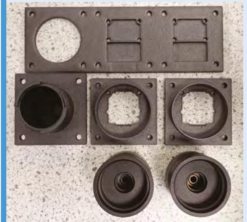
**02** The triplet mount was made from machined black anodised aluminium, resulting in improved precision and longevity over previous 3D-printed, non-triplet versions.
