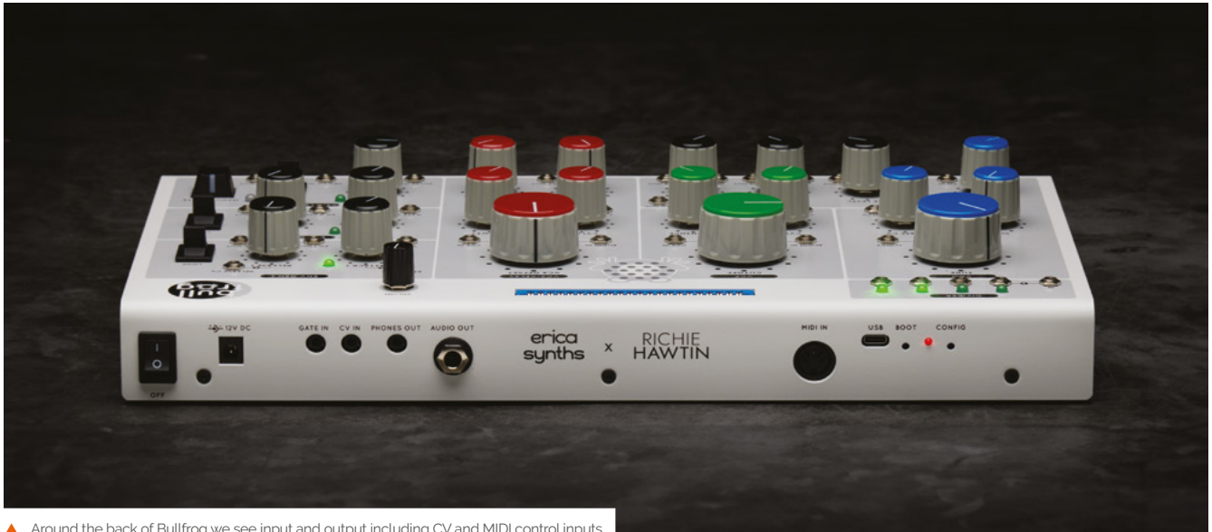
▲ Around the back of Bullfrog we see input and output including CV and MIDI control inputs
