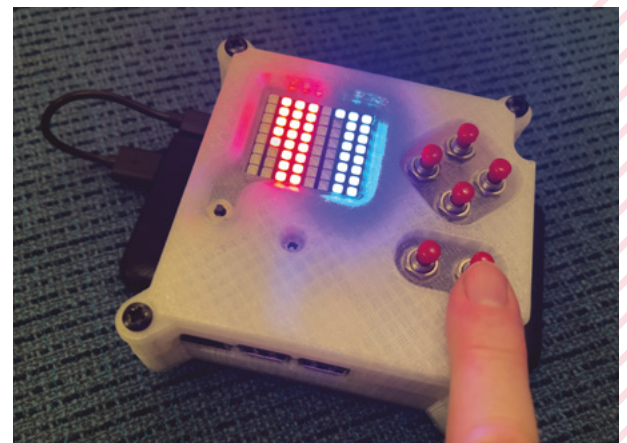
▼ This displays temperature and humidity, so during the demo people can figure out how the Sense HAT works
