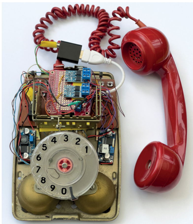
Figure 7 ♦ The two voltage converters are mounted on holders which are then stuck to the base of the phone. You can see them on each side just above the dial
