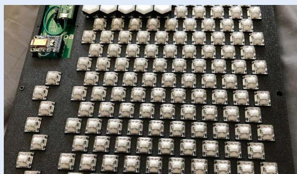
2. Solder the switches in place, then fire up the 3D printer and get to work creating a grid of tessellating hexagons.
