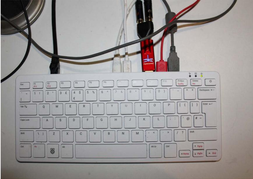
◀ Raspberry Pi 500's three USB ports are sufficient to connect both an audio capture device and a DAC, but if you have multiple instruments to connect, a more sophisticated audio interface makes sense and saves ports
