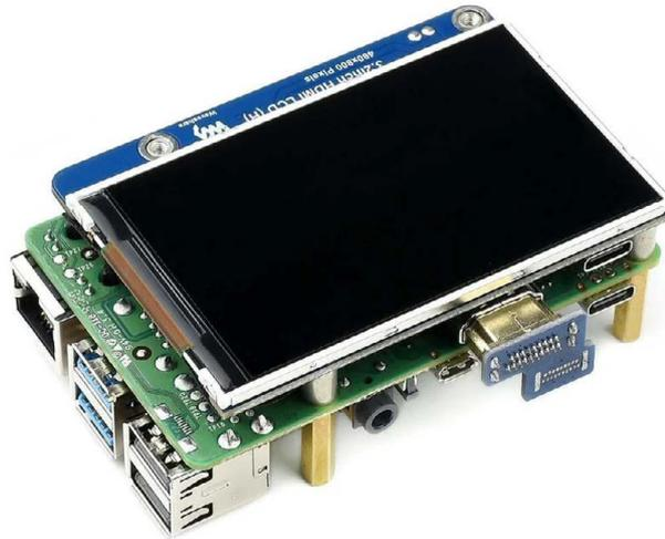
◀ You can mount this HDMI screen on the rear of a Raspberry Pi
