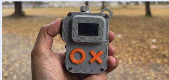
1. Although the device has a large orange O and X displayed on the front, these are not operational and they're merely aesthetic. The only actual button is a power one which is placed on the left side of the meter.
