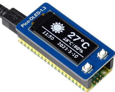
▲ This OLED screen mounts directly onto Pico's pins
