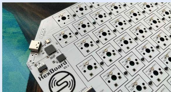
1. Design a custom PCB with all the ports you need, breakouts to the RP2040 module, and room for 140 mechanical switches.
