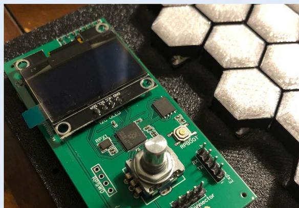
3. Meanwhile, create your own custom RP2040-based board – add this to the PCB to handle all the ins, outs, and programming.
