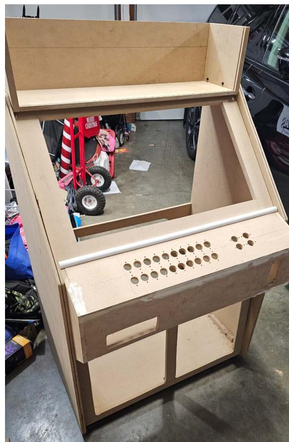
▲ The cabinet is completely modular. The marquee, monitor, button board and back panel bolt to the sides so it can be easily disassembled and moved if necessary
