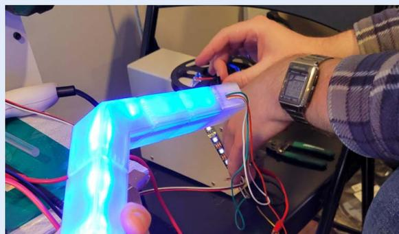
2. Downstall and install Hyperbian ([rpimag.co/hyperbian](http://rpimag.co/hyperbian)), a ready-to-use OS including the Hyperion LED controller. A string of addressable LED lights attached to Raspberry Pi's GPIO pins can be made to respond to the air hockey or gaming action.
