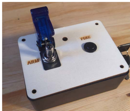
► Figure 5: Using a laser cutter to create a front panel for an existing plastic enclosure
