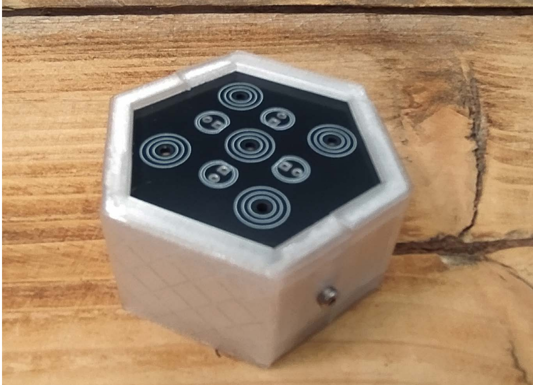
▲ Figure 9: A completed DIY enclosure with PCB front and rear panels; it would be simple to extend the case length in FreeCAD for larger projects
