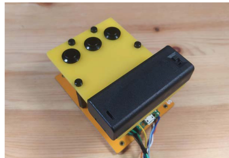
◀ Figure 6: Adding a small panel into which we mounted the buttons as a first attempt at a controller
