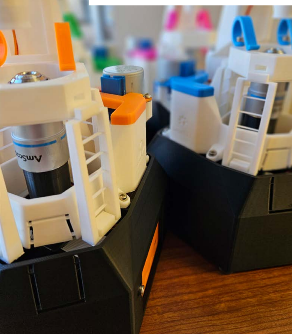
▼ Figure 1: The OpenFlexure Microscope is designed to flex to create movement needed for scanning microscopy
