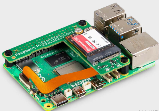
▲ M.2 HAT+ Compact mounted on Raspberry Pi 5
