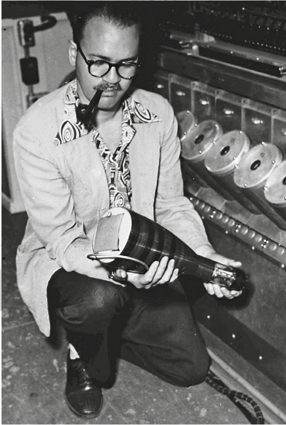
▲ James Pomerene working on the IAS machine, holding a Williams tube Image: Wikimedia Commons, CC BY-SA 4.0
