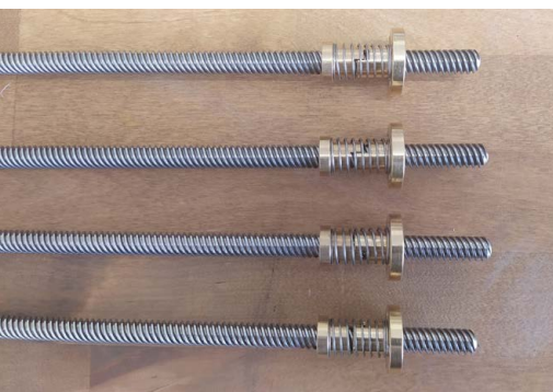
◀ Figure 1: Trapezoidal lead-screws will give us more accuracy than we probably need
