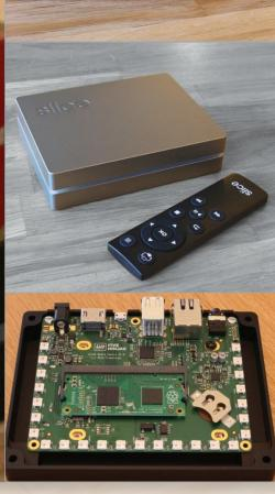
Right The anodised aluminium chassis houses a Raspberry Pi Compute Module, a real-time clock and can hold a slimline
