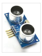
Left The HC-SR04 Ultrasonic Rangefinder. Cheap-as-chips sonar
