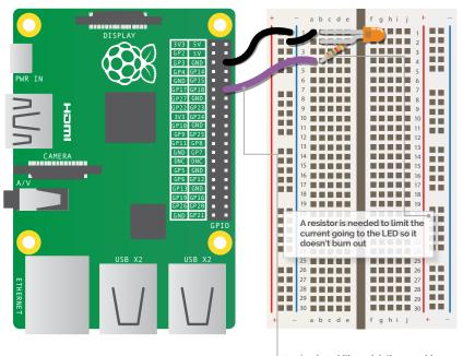
A pulse width modulation-capable GPIO pin is used to control the brightness of the LED
