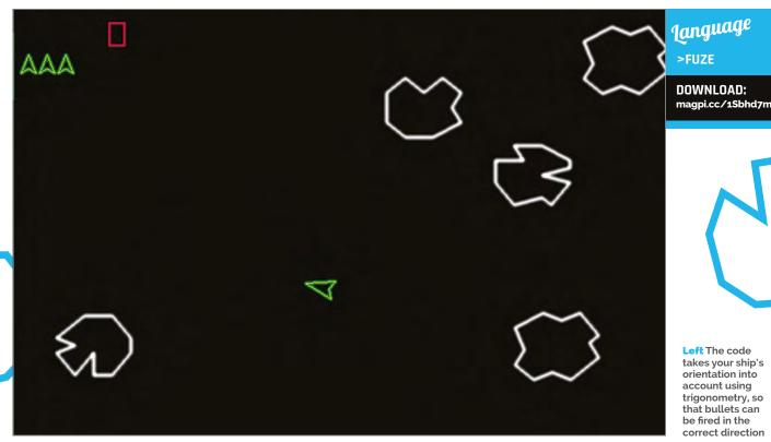
Left The code takes your ship's orientation into account using trigonometry, so that bullets can be fired in the correct direction
