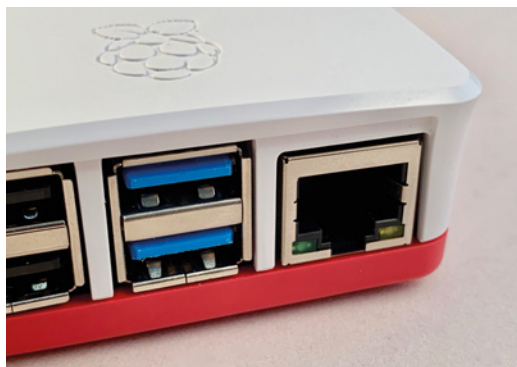
▲ USB 3.0 and full Gigabit Ethernet are essential to building a good Raspberry Pi NAS
