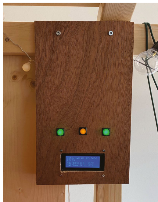
▲ The control box uses a simple LCD display for weather and time
