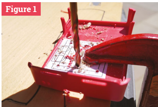
▲ Figure 1 Make sure you clamp the case, or carefully use a vice when drilling. Print out the template and stick it to the case
