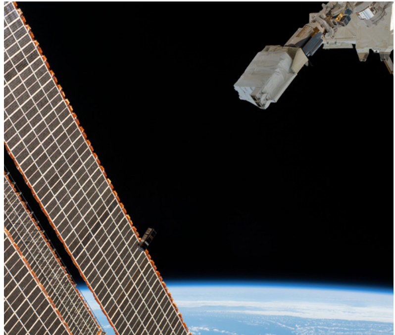
▲ A CubeSat from Singapore is ejected from the Japanese Small Satellite Orbital Deployer past the International Space Station's solar arrays. Credit: NASA
