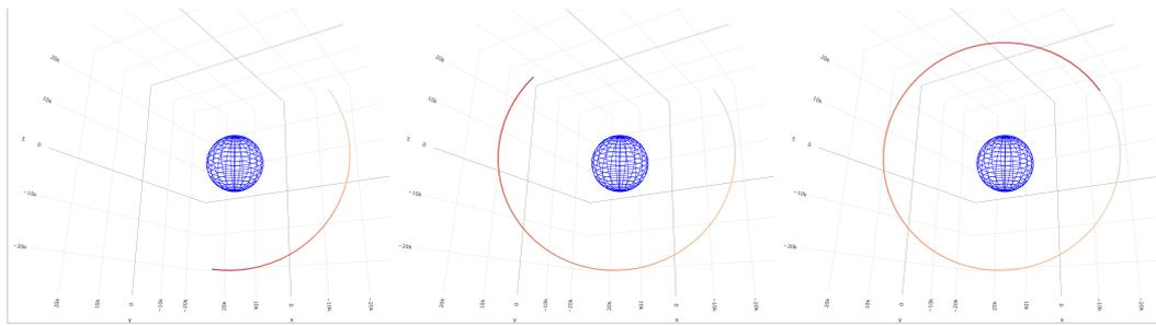
**Figure 3:** Trajectory of a GPS satellite calculated with the high-precision numerical propagator. It follows an almost circular orbit at an altitude of approximately 20200 km, which allows it to cover a larger portion of Earth at any given time.
