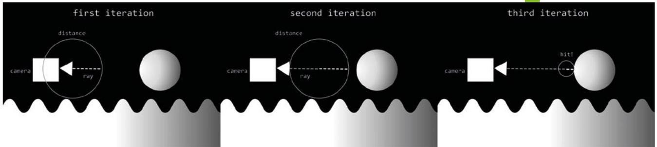
▲ Figure 2: Sphere tracing is how the ray travels using SDF functions. In the first two iterations, the floor is the closest object, but it doesn't hit the floor - it hits the sphere on the third iteration.
