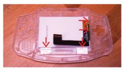
Figure 10: Be sure to orient the IPS panel as shown.
