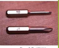
Figure 3: The Y0 bit is primarily used on the exterior of most Nintendo consoles to deter consumers from getting inside. Internal screws are typically Japanese International Standard (JIS) - see box on page 55 for more info.
