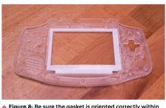
Figure 8: Be sure the gasket is oriented correctly within the LCD cubby. The thinner border is on the left and the thicker border is on the right.
