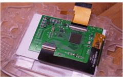
Figure 13: IPS panel connected to the driver board.
