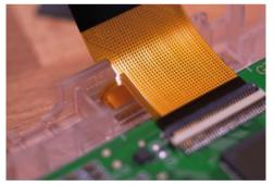
Figure 15: The touch sensor should be folded over facing towards the front shell.
