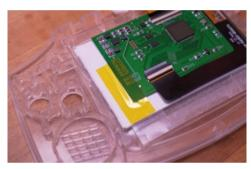
Figure 14: Taping the driver board to the back of the IPS panel keeps it from shifting around and makes the installation easier.
