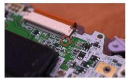
Figure 5: Marking to indicate whether you have a 32 or 40 pin motherboard. This will dictate which ribbon cable you'll need for the backlight kit.
