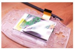
Figure 16: Putting the protective film over the driver board will prevent shorts when you put everything back together.
