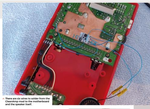
have to solder two extra lengths of wire from the mod to the speaker in order to cover the gap – arguably the fiddliest bit of the modding process. Still, I managed to get the whole job done in about 20 minutes, and made sure my extended speaker wires were nicely protected by wrapping a bit of Kapton tape around each one (you may want to use heat shrink tubing here – something I don't currently have in my tool-kit).
