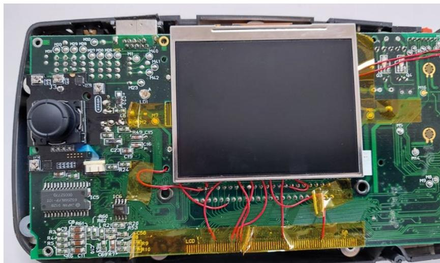
to keep a Game Gear from dying – that is, replace all the capacitors, and maybe install a modern LCD screen – then you shouldn’t have too much trouble installing the RetroSticks. The device lies directly on top of the contacts where the D-pad would typically sit, and there are six contact points where the thumbstick is soldered onto the Game Gear’s motherboard.
