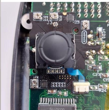
▲ The RetroSticks GG soldered in place. Those screws around the edge of the device are used for calibration.
