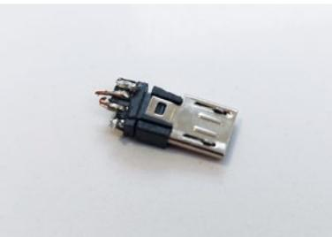
^ **Figure 4:** The wires from the controller need to be soldered to the connector like this. If you don't have a set of helping hands, taping the connector to a lid like this helps keep it still.
