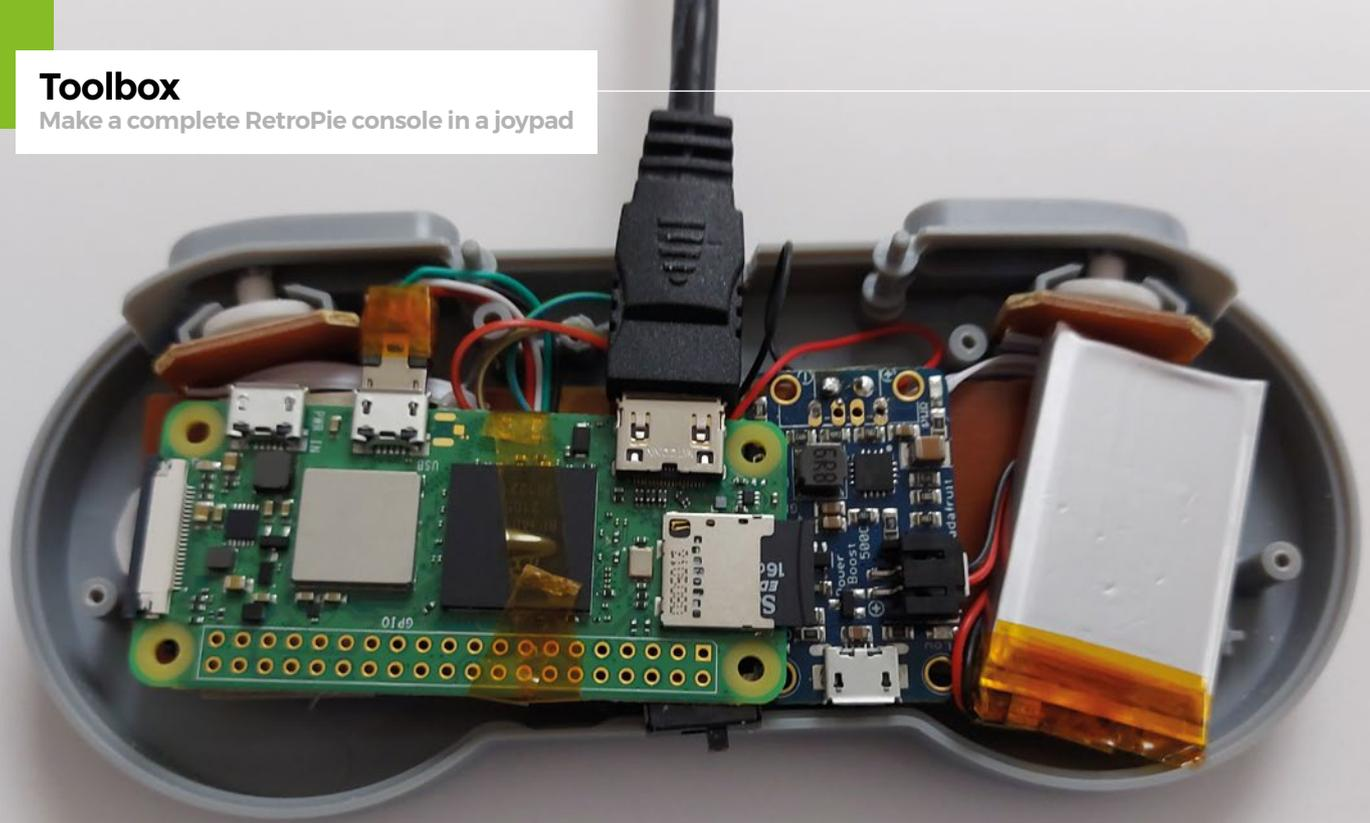
▲ Figure 10: Here's how all the parts need to fit inside the controller.
