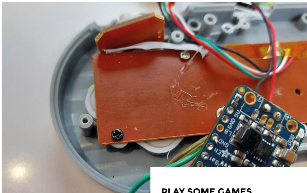
◀ **Figure 14:** To keep our buttons feeling nice and firm, we added a couple of small screws to the controller's board.
